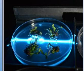
A 488nm wavelength laser scans over the area of a Petri dish to detect GFP, chlorophyll, and other fluorescence signatures in the sample.
