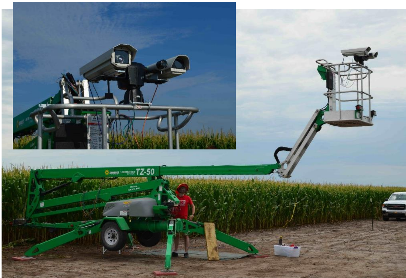
3 camera set up VNIR, NIR and Thermal
