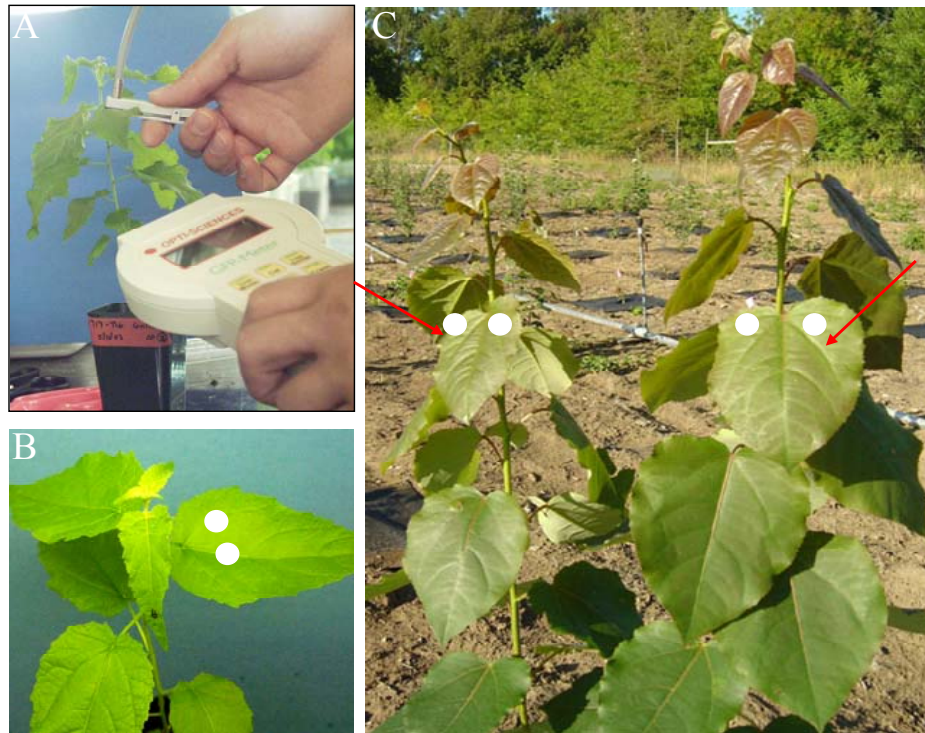
Fig. 2. 3. Measurement of GFP fluorescence with a GFP-meter (A) in the greenhouse (B) and field (C). White spots on the leaves (B & C) are approximate spots that were measured for GFP expression. Red arrows indicate two leaves from two shoots of a plant sampled for fluorescence measurements.
