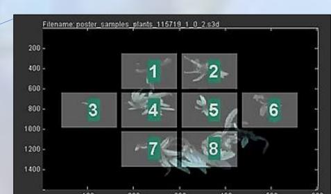
A custom grid overlay system was developed so that KemoQuant™ will recognize tissue explants on a Petri dish and output their data individually.
