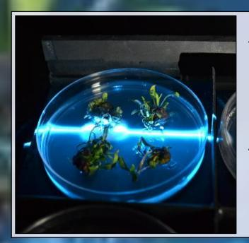
A 488nm wavelength laser scans over the area of a Petri dish to detect GFP, chlorophyll, and other fluorescence signatures in the sample.
